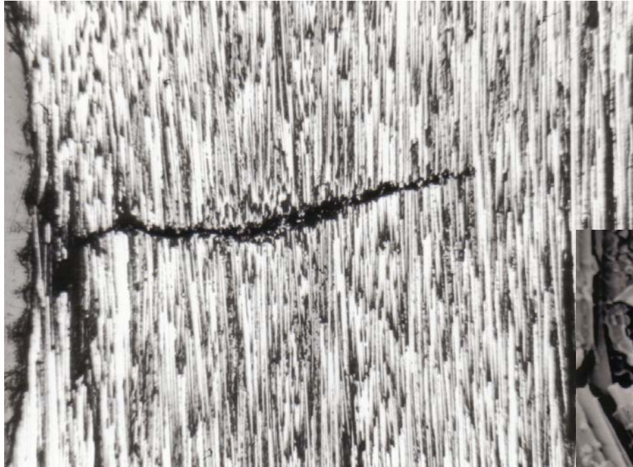
Fibre microbuckling in a T800/924C Laminate (6 \mu m fibre diameter)
