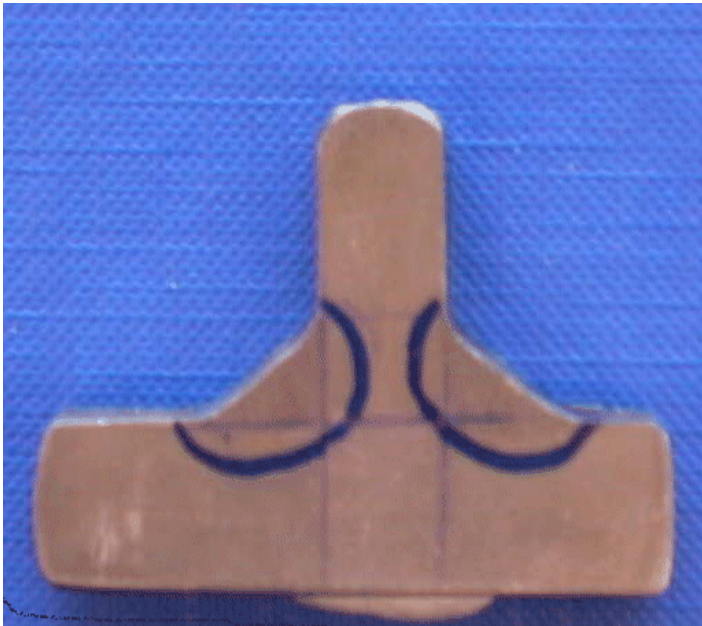
T-junction section, highlighting HAZ region
